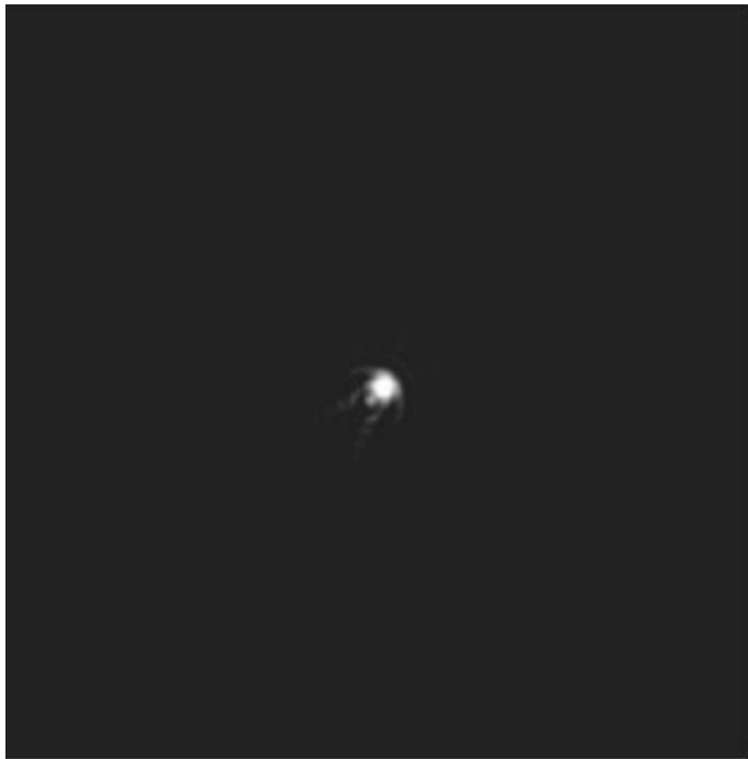
CT-image of wire (phantom measurement)
