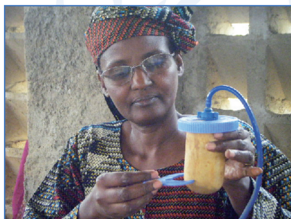
Figure 6 : Woman monitoring the thickness of the filter element of a Tulip Siphon filter Photo: 300in6
